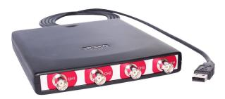
TiePie engineering introduces the Handyscope model HS4, a portable and compact MOST (Multimeter, Oscilloscope, Spectrum analyser and Transient recorder). As four channel measuring device with a 50 MHz sample frequency, a 12-16 resolution and 128 KSamples memory per channel, the Handyscope HS4 is the first four channel MOST in the world which can be connected to a PC (USB2.0 and USB 1.1 compatible), without external power supply.
