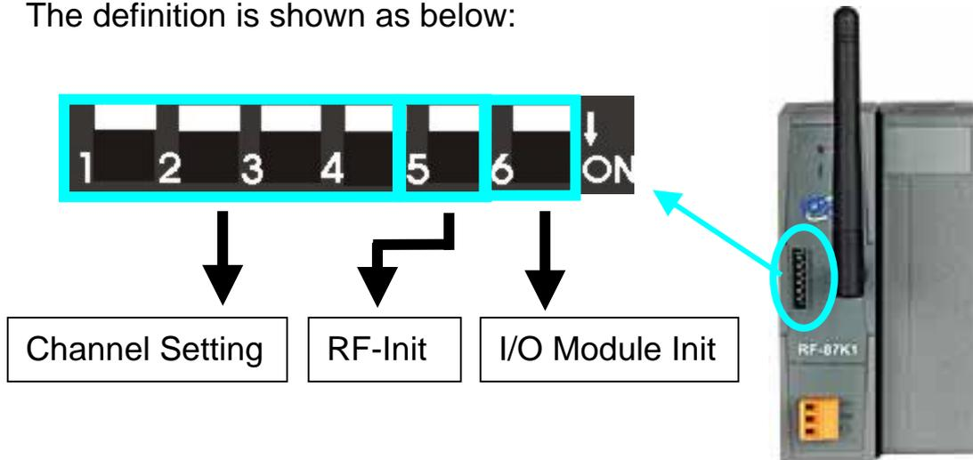
**Channel Setting:** The first four bits allow the user to select any of the sixteen channels. Refer to Table 5.3 in Section 5.3 for the relevant settings.
