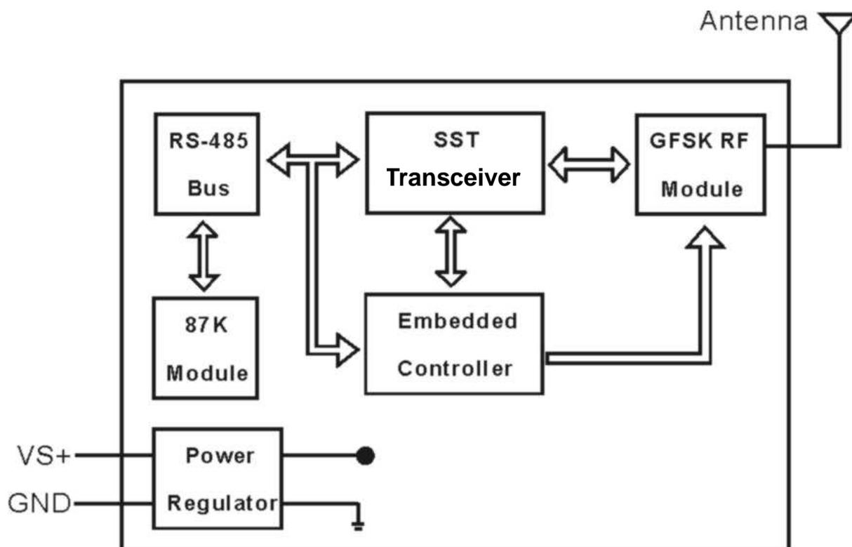
RF-87K series modules contain two elements. The first is the RF module (for radio communication) and the second is the I-87K module slot (for data acquisition).
