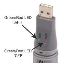
One LED is for temperature measurement, the other is for RH. Each is clearly marked on the logger. To save power, the status indication alternates between the two channels every 10 seconds. So first you will see the status of the temperature logging; 10 seconds later you will see the status of the RH logging and so on.
