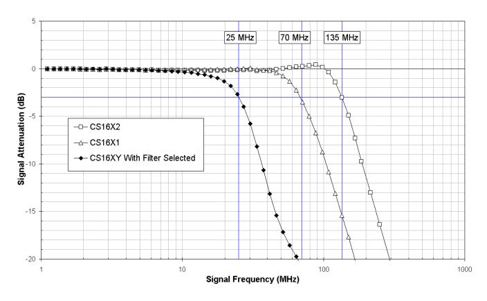
Note: Typical Frequency Response curves above taken on  $\pm 500$  mV input range with on with  $50~\Omega$  termination with DC coupling. In AC Coupled mode, the lower -3 dB cutoff frequency is 200 kHz.
