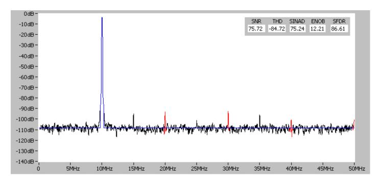
Frequency spectrum above taken on a Razor CS1641 on its  $\pm 500$  mV input range with  $50 \Omega$  termination and DC coupling.
