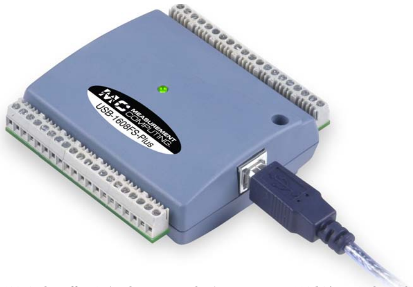
The USB-1608FS-Plus offers 8 simultaneous analog inputs at up to 100 kS/sec per channel (400kS/sec overall), 8 digital I/O, and one event counter input.
