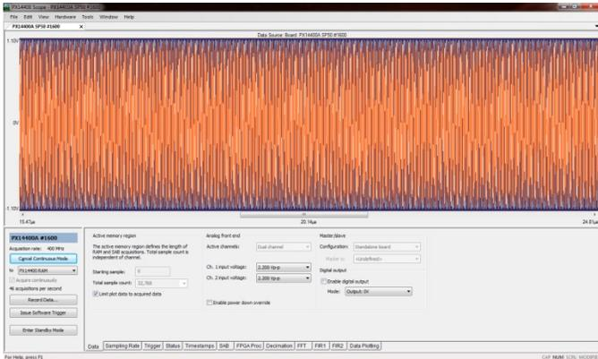
The PX14400 Scope App software is a virtual oscilloscope application that allows the operator to view or edit all digitizer hardware settings as well as record and display acquisition data.
