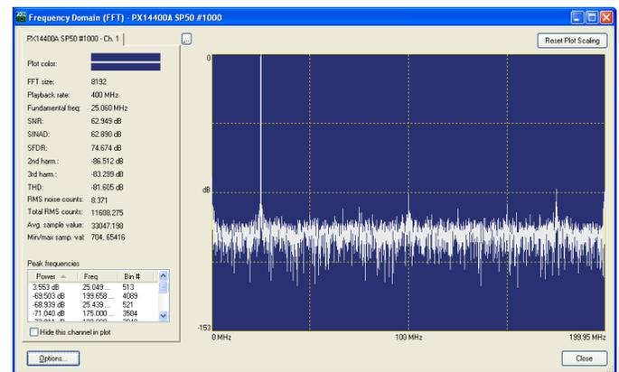
The FFT window is divided up into two regions. The left side is a tab control that contains various FFT and time-domain statistics. There is one tab for each channel of data. The right side contains the frequency domain plots of all channels.
