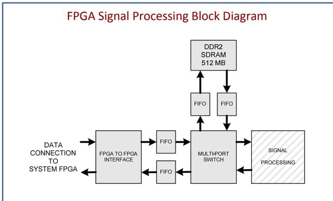
When FPGA processing is enabled, acquired data is transferred from the System FPGA to the Signal Processing FPGA where the targeted signal processing routine is conducted. The resulting processed data output is then transferred back to the System FPGA, which can then stream the resulting data to the host PC system via the PCIe interface with PCIe Buffered Acquisition mode.
