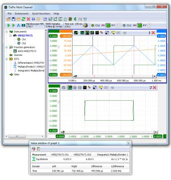
This measurement determines the area of an XY graph, using multiplying, integrating and differentiating I/O's. The area is indicated in the Value window:  $16 \text{ V}^2$ .
