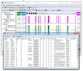
The various serial protocol analyzers of the Handyscope HS5 can be used to analyze and debug serial data buses. The data is displayed in an elaborate table with information on the serial data. Locating "wrong" data packets has become very easy. For each developer or service technician this is a welcome option. Protocol analyzers for CAN bus data, I<sup>2</sup>C communication and various other serial data communications are available.
