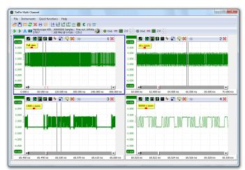
Shown is a 30 million samples long measurement. The same signal is shown four times in different zooming factors, the lower right graph shows just 0.01 ms of the total 300 ms, a zoom factor of 30000. It still provides enough detail for accurate signal analysis.
