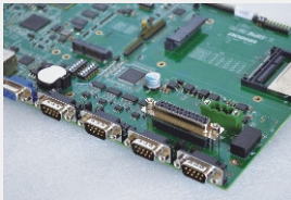
8KV electrostatic protection, TVS 600W surge protection, 2500VDC isolation serial magnetic coupling
