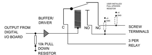
not randomly open or close on power-up. Also, buffer/ drivers on board accept signals from simple 8255 type digital I/O boards.
